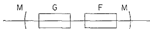
Fig. 1. The mirrors M define the resonant frequencies of the cavity. Inside the cavity is both a region of gain G (population inversion) and a region of fluctuation F (chemical reaction).
