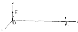
Fig. 2. The cavity corresponds to 0 < z < L and the electric field is parallel with the x axis.
